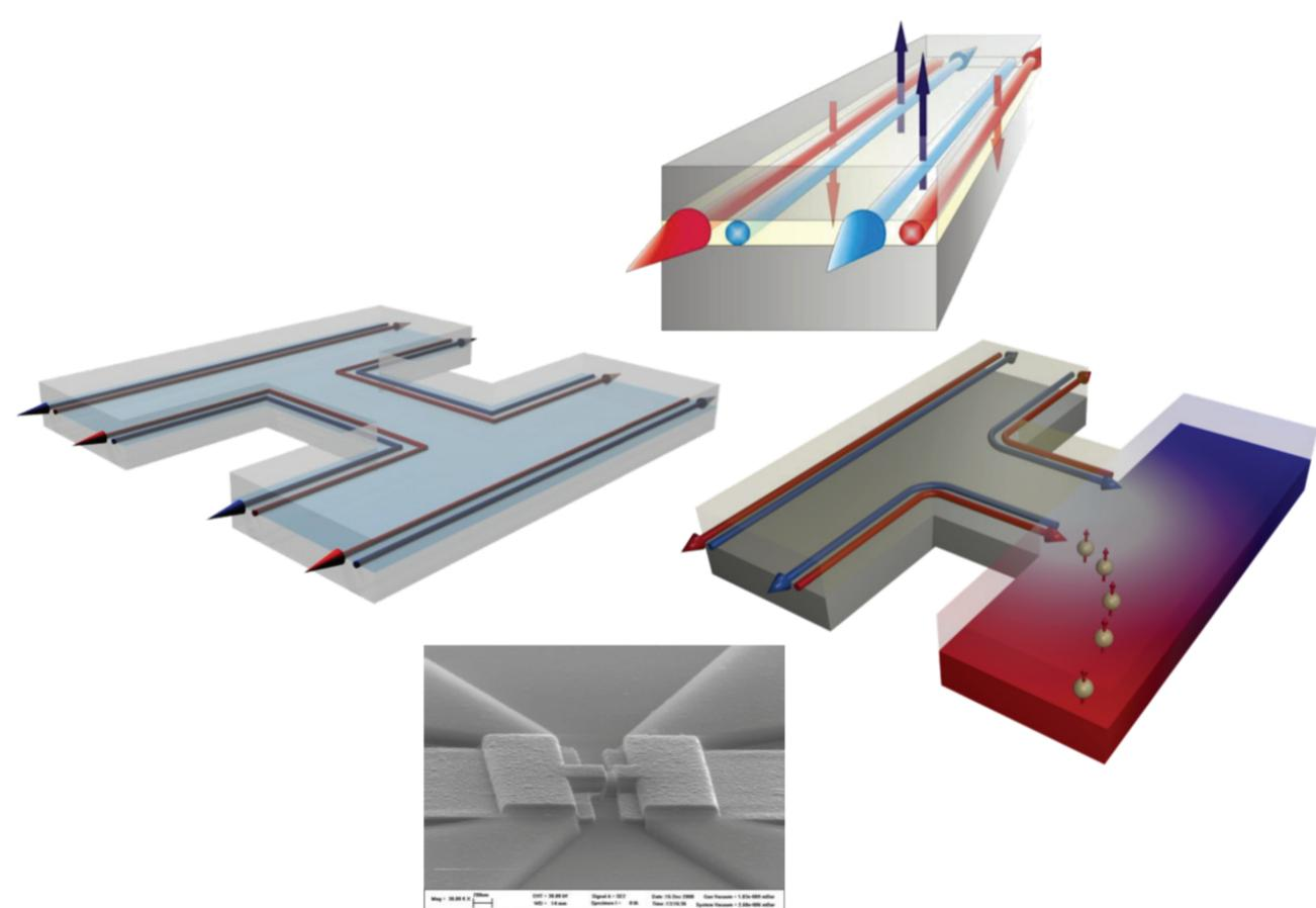
The most straightforward way to do so is by growing a quantum well with (Hg,Cd)Te barriers. Such structures exhibit the quantum spin Hall effect, where a pair of spin polarized helical edge channels develops when the bulk of the material is insulating.
