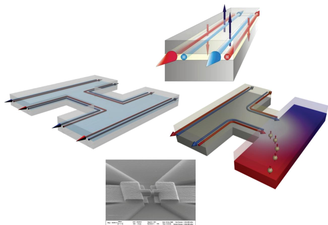
The most straightforward way to do so is by growing a quantum well with (Hg,Cd)Te barriers. Such structures exhibit the quantum spin Hall effect, where a pair of spin polarized helical edge channels develops when the bulk of the material is insulating.
